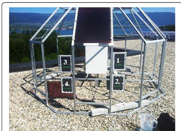
**Fig. 7** Solar monocrystalline panels test rig for self-cleaning tests
