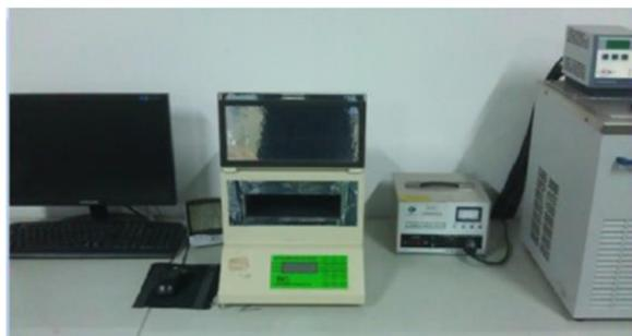
**Fig. 5** Laboratory measurement meter of thermal conductivity
