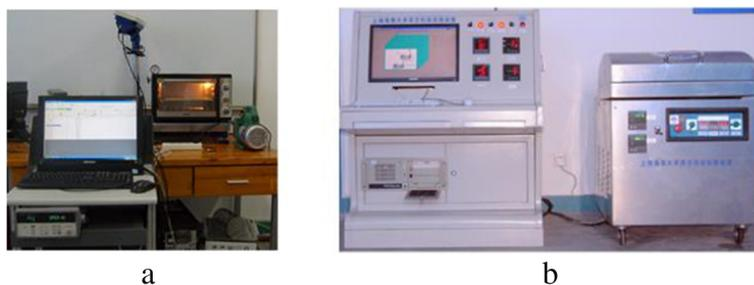
**Fig. 4** The VIPs making equipments: (a) The vacuuming and heating alternation pre-treating equipment; (b) program controlling VIPs making machine
