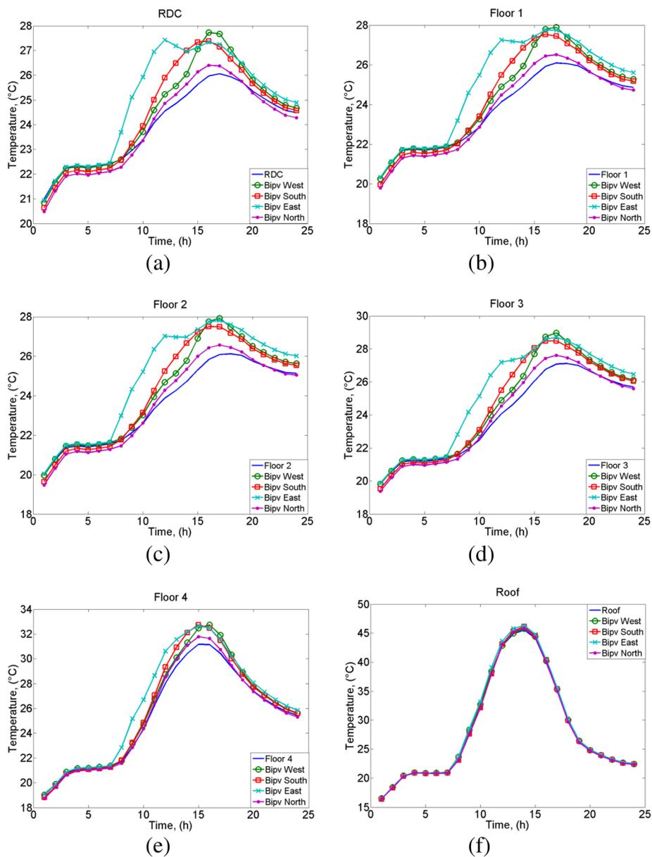
**Fig. 6** Hourly temperature variation of indoor air of the main floor building (a), floor 1 to 4 (b) – (e) and roof (f) for BIPV facade integration with building orientation
