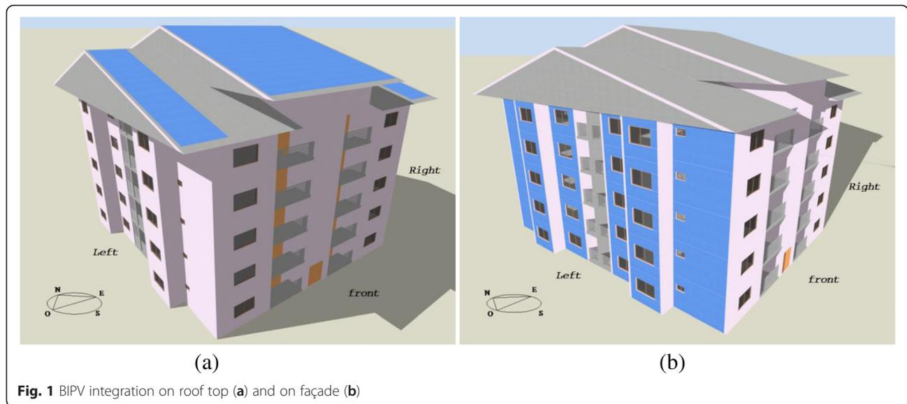
**Fig. 1** BIPV integration on roof top (a) and on façade (b)
