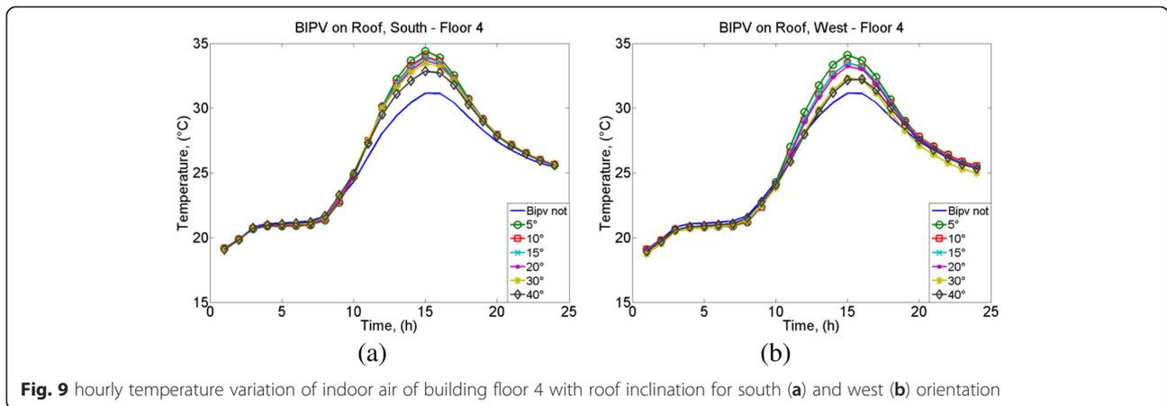
**Fig. 9** hourly temperature variation of indoor air of building floor 4 with roof inclination for south (a) and west (b) orientation
