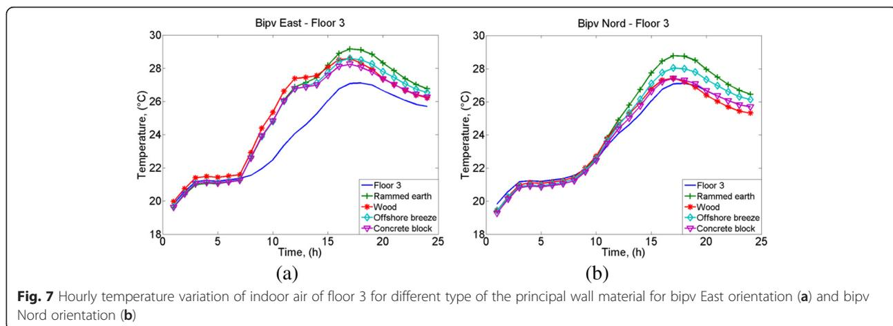
**Fig. 7** Hourly temperature variation of indoor air of floor 3 for different type of the principal wall material for bipv East orientation (a) and bipv Nord orientation (b)
