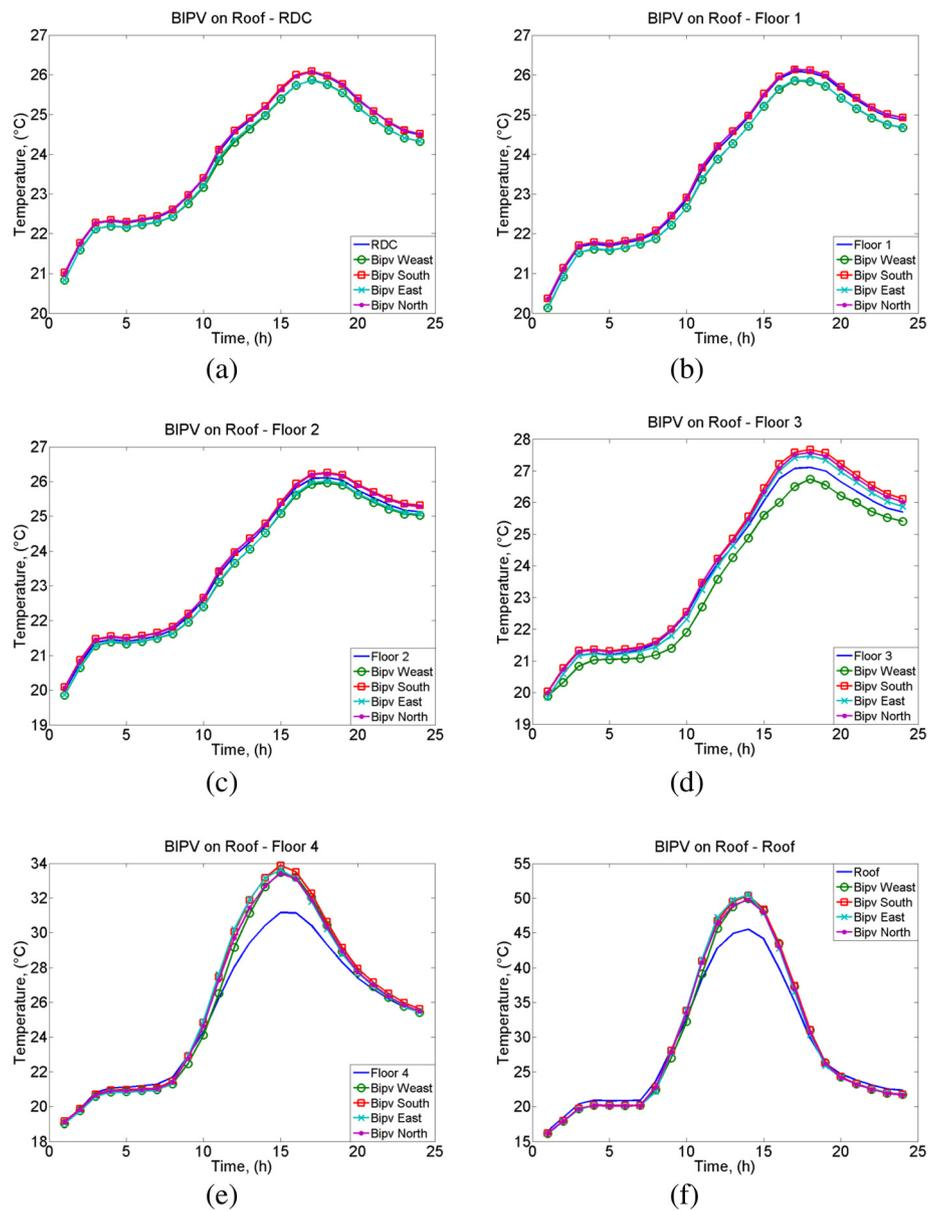
**Fig. 8** Hourly temperature variation of indoor air of the main floor of building (a), floor 1 to 4 (b) – (e) and roof (f) for BIPV roof integration with building orientation
